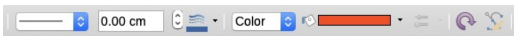
Figure 211: Drawing Object Properties toolbar – some controls are available for setting default properties
