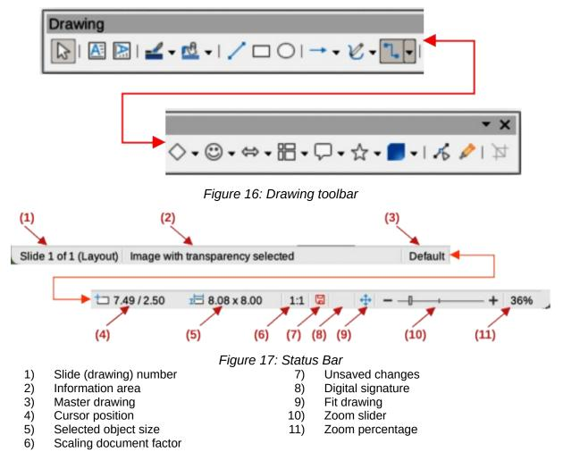
Some tool icons on the Drawing toolbar change shape according to the last tool used from the selection of available tools. Each tool that has a triangle ▼ next to the tool icon indicates that more tools are available. See "Drawing geometric shapes" on page 43 for information on the available shapes.
