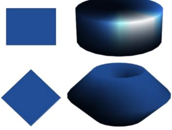
Figure 174: Example of 3D conversion using rotation
