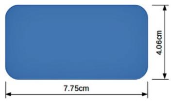
Figure 29: Example of dimension lines for an object
