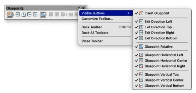
Figure 8: Example of Visible Buttons
