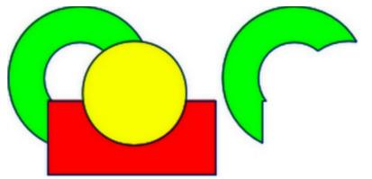
Figure 126: Example Of subtracting objects
