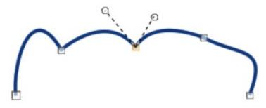
Figure 308: Example of a corner point
