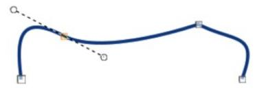
Figure 309: Example of a smooth transition point
