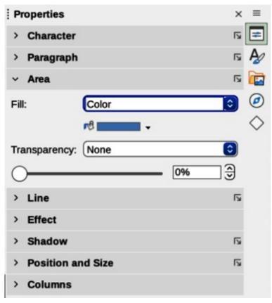
Figure 299: Area panel in Properties deck on Sidebar
