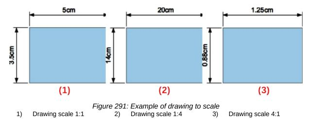
An increase in scale (for example 1:4) allows large objects to be drawn that would not fit into the paper size for a drawing. A decrease in drawing scale (for example 4:1) allows small objects to be drawn accurately at an increased size and make them easier to understand. Examples of drawing to scale are shown in Figure 291 where all three rectangles are the same size in the drawing.
