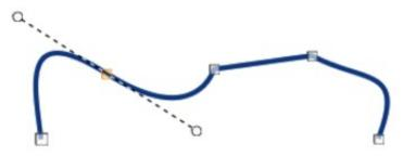
Figure 310: Example of a symmetric transition point
